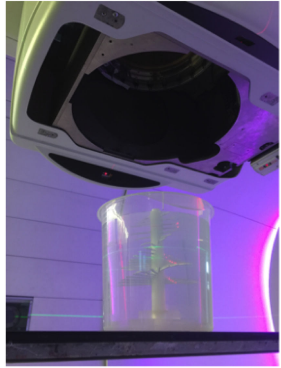
(b) Holder positioned in water-phantom on treatment couch
