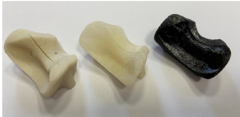
Figure 6. Cutting guides printed by FDM in PLA ( left ), HTPLA ( center ), and nylon ( right ).
