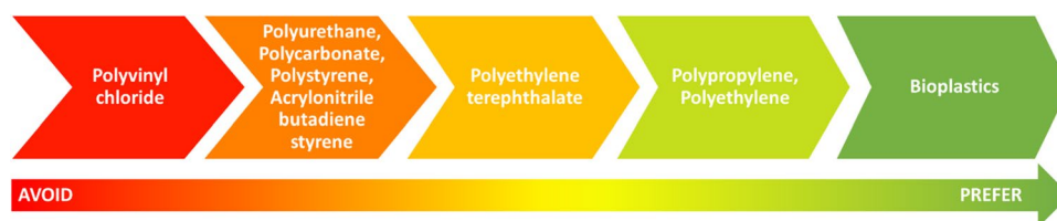
Fig. 4 Spectrum for the recommended usage of plastics considering environmental sustainability (Adapted from Arikan and Ozsoy 2015). Bioplastics are the most preferred followed by polypropylene, polyethylene and polyethylene terephthalate, polyurethane, polycarbonate,
