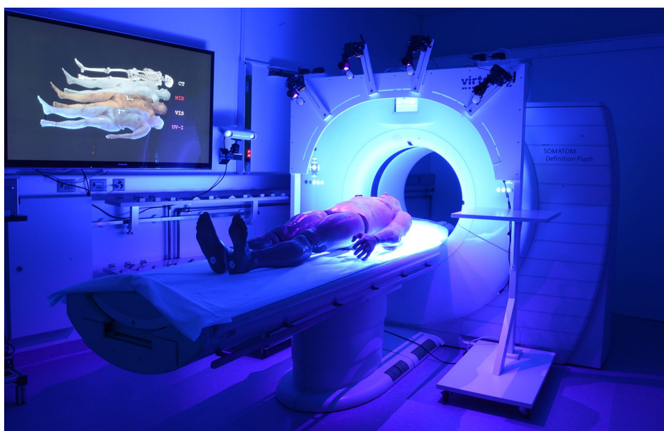
Fig. 1 Photo of the multispectral imaging setup in front of the CT gantry. In this photo, the multicamera rig is equipped with UV light sources and yellow lens filters with 50% transmission at 460 nm
