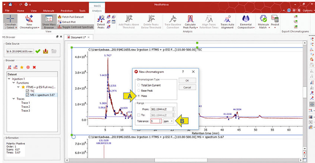
Fig. 3. Layout of MestreNova application when mass browsing to produce an extracted ion chromatogram (EIC). Arrows indicate commands for selecting type of chromatogram (a) and tolerance range (b)
