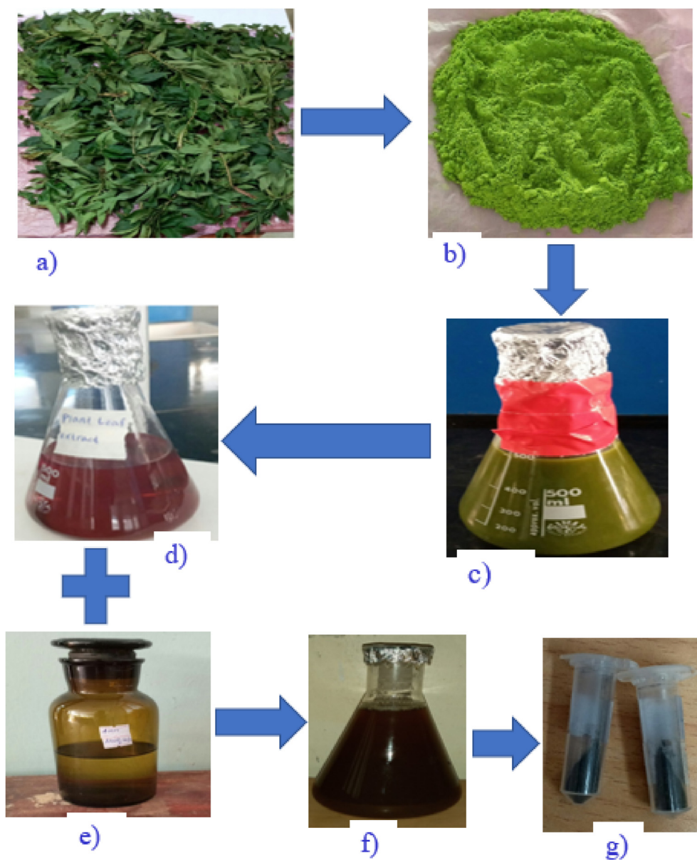
Figure 3. Green synthesis of AgNPs from HAPLE after incubation at 40 °C for 90 min, and colour change observation: a) Hagenia abyssinica plant leaf; b) Hagenia abyssinica plant leaf powder; c) Macerated Hagenia abyssinica aqueous plant leaf extract before filtration; d) Hagenia abyssinica aqueous plant leaf extract after filtration (dark-red); e) 4 mM aqueous AgNO 3 solution; (colorless); f) Colloidal AgNPs (dark-brown) and g) Powdered AgNPs.
