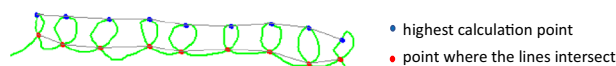
Figure 3. Extracted from the handwriting analysis device (Elian Research software, Version 4.2, http://www.seldage.com ) for the copy of a line of cycloid loops. Each point forming the line of loops and the highest point of the loop, the intersection point are recorded for the calculation of the following features: total drawing length, average length per stroke, drawing width, drawing height, degree of inclination of the line, height of the loops, spacing between loops, number of loops, number of strokes, total drawing time, effective drawing time, number of on-paper pauses, number of in-air pauses, number of velocity peaks, average and maximum velocity.
