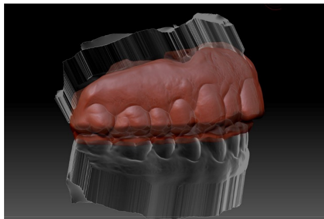
Figure 4. Design of the inner layer (red) (2 mm) using “inflat” tool in the Zbrush software.
