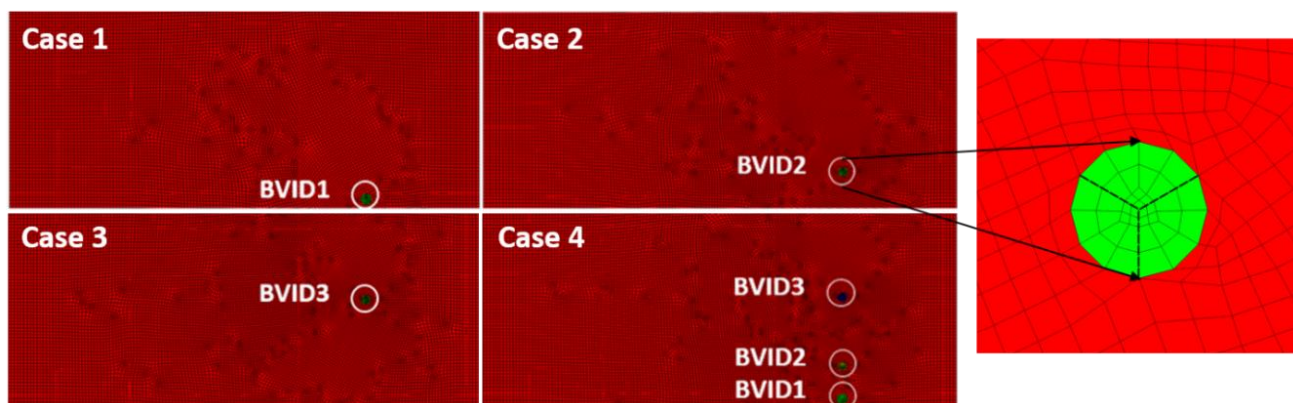
Figure 3. SEM_GFRP model cases studied.
