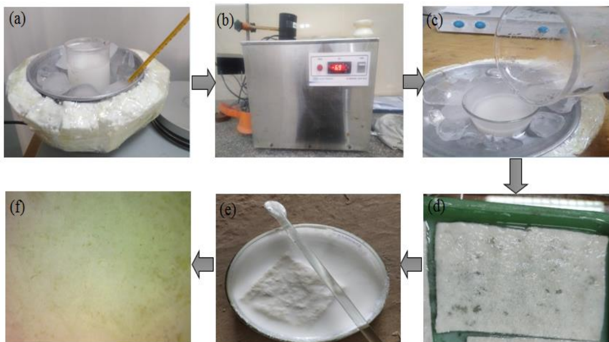
Figure 1. The process flow of cellulose hydrogel reinforced with nonwoven cotton: (a) MCC solution preparation at 5\text{ }^\circ\text{C} ; (b) NaOH solution preparation at -6\text{ }^\circ\text{C} ; (c) mixing of NaOH/MCC solution; (d) nonwoven fabric dipped in MCC hydrogel; (e) sample dip in \text{TiO}_2 solution; (f) cellulose hydrogel-reinforced with nonwoven cotton fabric.
