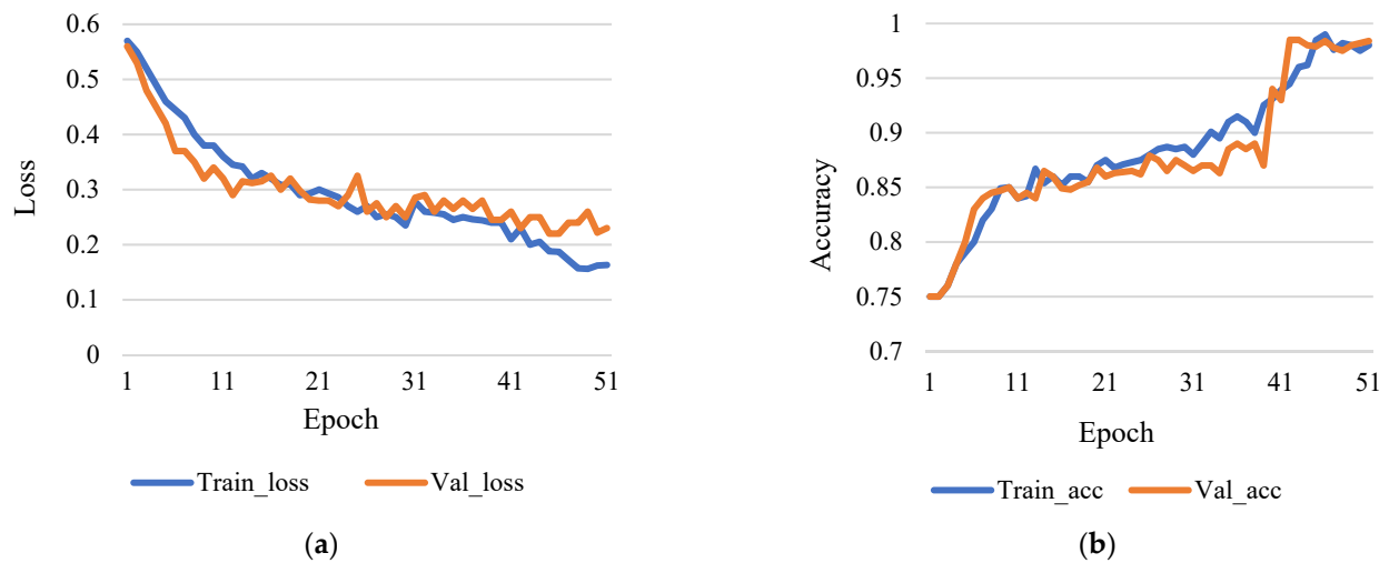
Figure 8. (a) Training loss vs validation loss (rate of learning 0.01 and epoch 50). (b) Training accuracy vs validation accuracy (rate of learning 0.01 and epoch 50).
