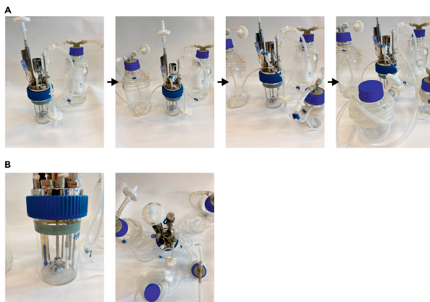
Figure 5. Schematic overview of the assembly of bottles to the DASbox bioreactor
