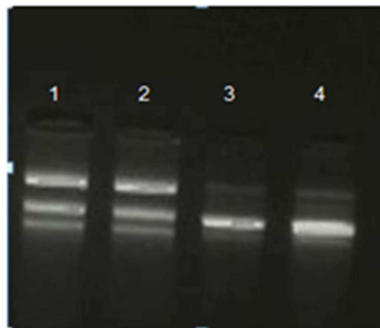
Fig. 5 Agarose gel retardation assay of pDNA complexes with the modified MSNs in various N/P ratios (0.2, 0.5, 1, 2, and 5) in comparison to free pDNA
