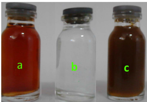
Fig. 1 Colour changes in the reaction solution (a) Aqueous extract of thyme leaf, (b) Aqueous solution of 1 mM AgNO 3 , (c) Reaction mixture (plant extract + AgNO 3 solution) after AgNPs formation
