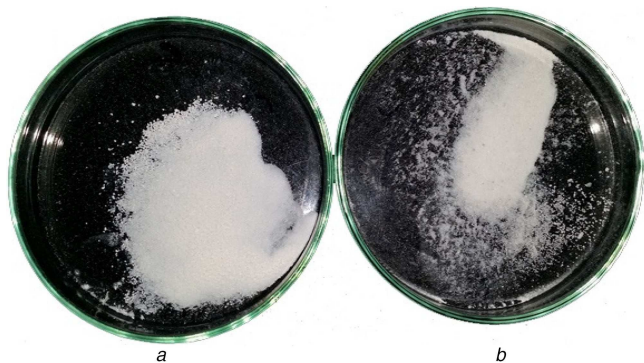
Fig. 2 White powdered Si-NPs (a) Prepared from plant extract, (b) TEOS and CTAB, prepared from plant extract and TEOS
