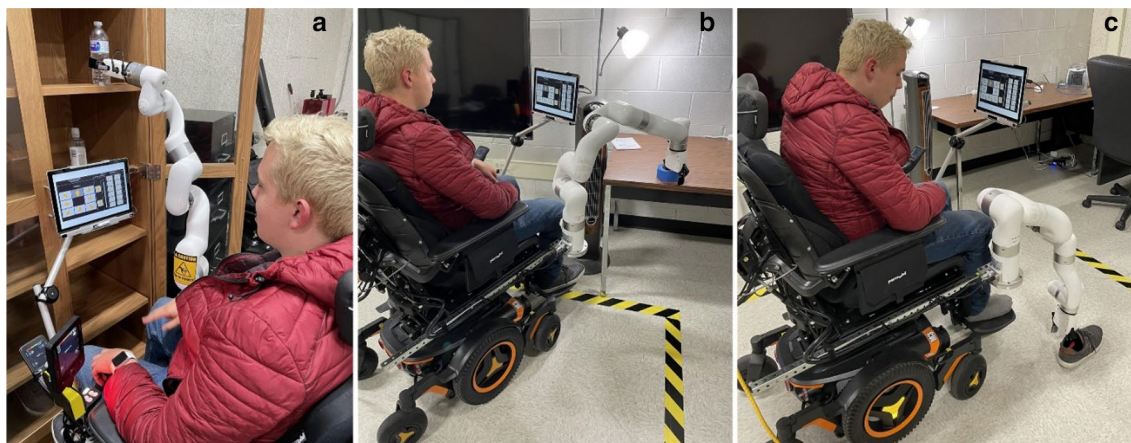
Fig. 12 Activities of daily living experiment with a healthy subject. From the left, a getting something from the upper shelf, b picking objects from the table, and c picking things from the ground
