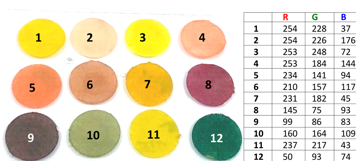
Figure 3. (Left) Filter paper disks coated with sensory polymers after spraying an acid solution of sodium nitrite (0.1 g \text{NaNO}_2 , 25 mL water, 2.5 mL HCl (37%)) and an aqueous solution of NaOH (1 M). (Right) RGB color definition parameters for each disk.
