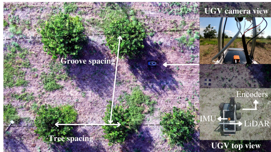
Figure 8. The mobile 3D LiDAR mapping system into the citrus crop.
