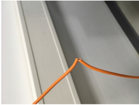
(a) Sample in the dataset for a red broken cable used for electrical circuits.
