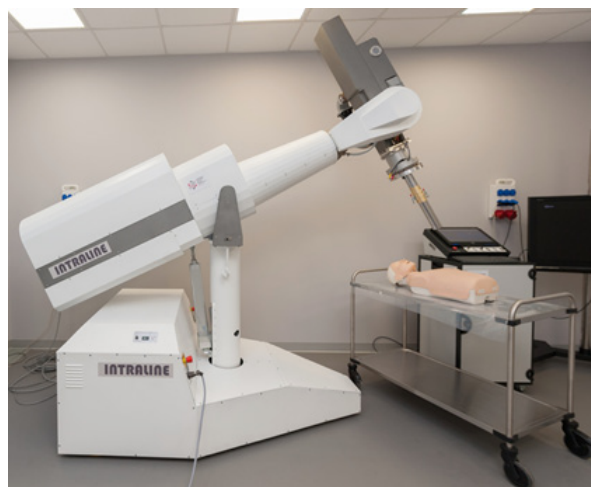
Figure 1. General view of the mobile intraoperative linear accelerator which being developed by the National Centre for Radiation Research
