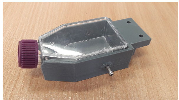
Figure 5. T-25 cell culture bottle placed in the holder. The holder was specially designed and printed in the 3D technique
