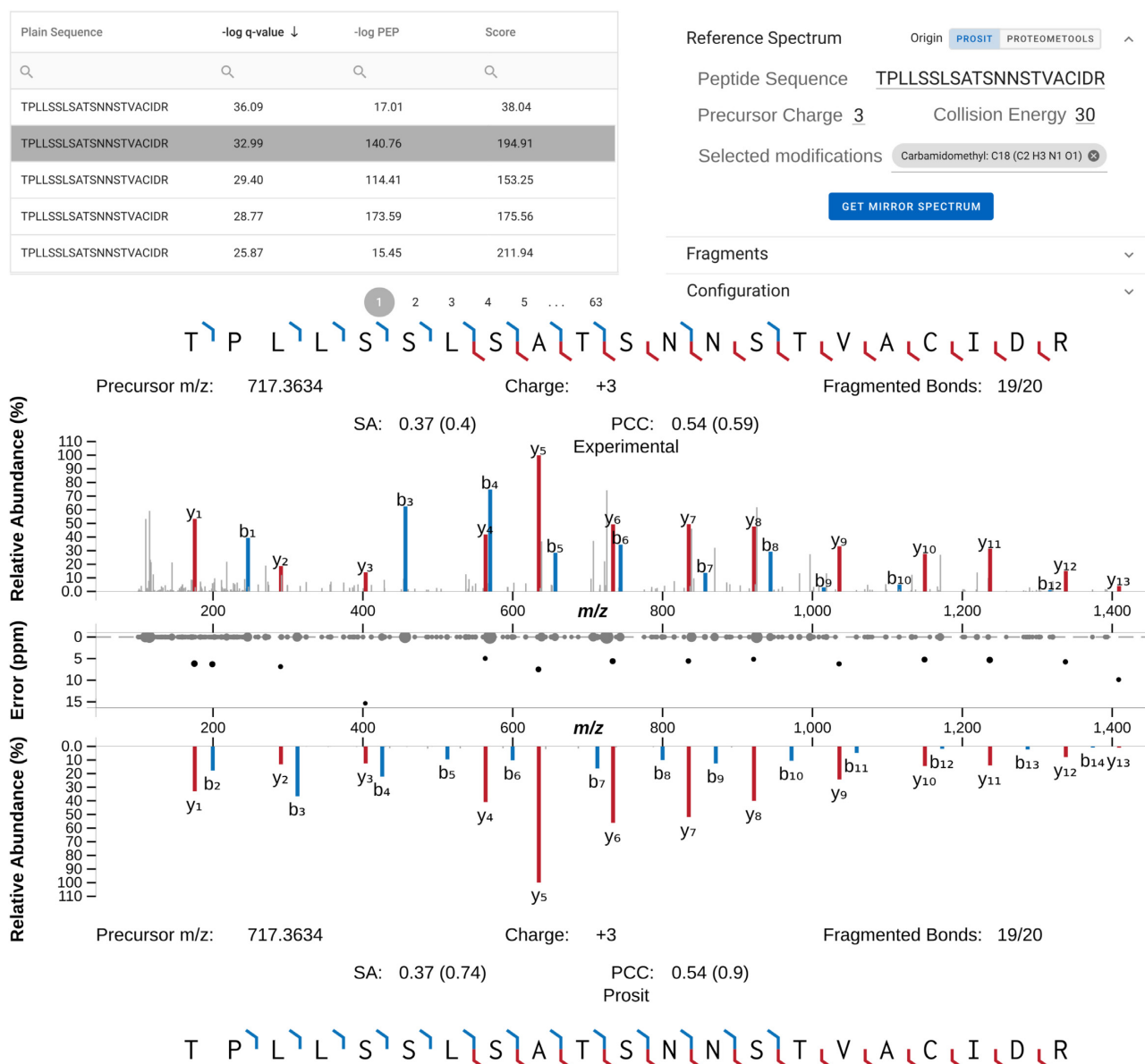
Figure 5. Spectrum viewer. The spectrum viewer (bottom) visualizes the selected peptide spectrum match from the table in the top left. The configuration element on the top right can be used for, but is not limited to, retrieving reference spectra depicted in the mirror view to the bottom. Reference spectra can be generated in real-time by Prosit or requested from ProteomeTools. In between the experimental and reference spectrum, the alignment error between an observed and reference peak is shown in parts-per-million (ppm). The spectral similarity between the experimental and reference spectrum is measured by calculating the Pearson correlation (PCC) and normalized spectral contrast angle (SA). The measures inside the brackets show the result of this comparison when taking either the peaks of the experimental or reference spectrum into account whereas the values outside the brackets show the measures calculated taking all peaks from both spectra into account.
