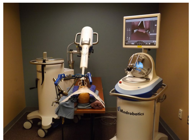
Fig. 1 The Medrobotics FLEX™ System and experimental setup. The flexible endoscope device can be seen in white and is operated by the surgeon from a computer station fitted with a haptic drive control. There are also two working ports where various surgical instruments can be brought into the operating field and are directly manipulated by the surgeon standing at the head of the bed. This setup allows for flexible access into the upper aerodigestive tract with one primary scope. The airway mannequin head can also be seen secured to the table
