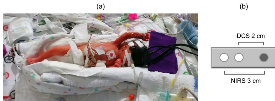
Figure 5. (a) Premature infant with optical probes secured to the forehead and a phototherapy eye shield, (b) schematic of probe holder showing the position of the NIRS (3-cm SDD) and DCS (2-cm SDD) sources and the common detection location (shaded circle). Probe holder was 5 \times 2 \times 1 cm.
