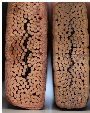
Figure 3. Comparison between two dummy cables after Cu thermal spraying. On the left, the cable was coated as free-standing. On the right, an Al fixture was constraining it during coating.
