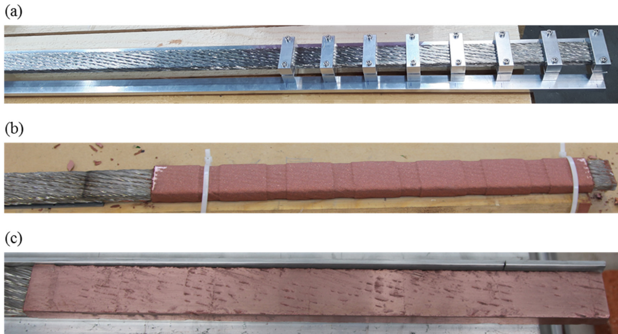
Figure 4. Superconducting cable before Cu arc spraying (a), after Cu deposition (b) and milling of the surfaces (c).
