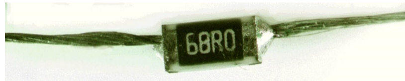
Figure 4. SMD integrated E-yarn.
