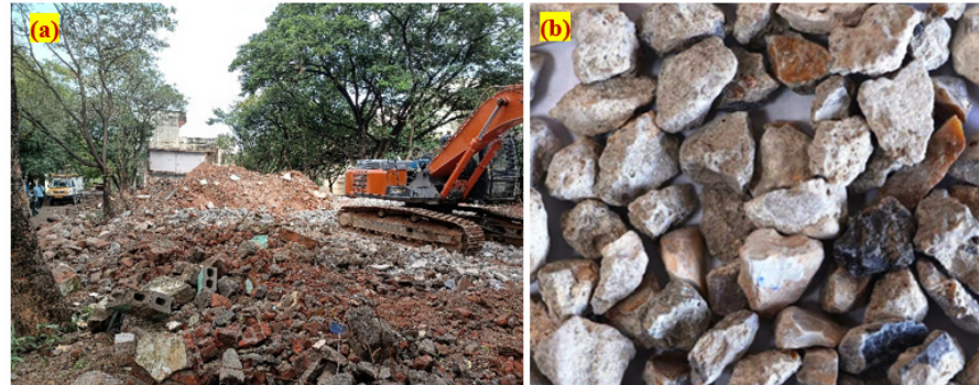
Figure 1. Details of RCA: (a) source (b) appearance of recycled aggregate.
