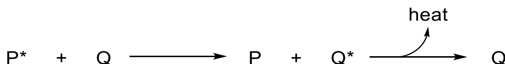
Figure 5. UV absorbers act as quenchers for the excited state energy of polymers. * Represents the excited state.
