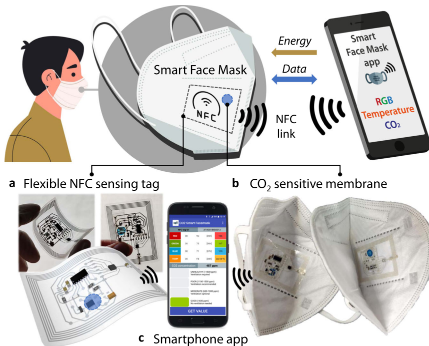
Fig. 1 Overview of the NFC-based smart facemask for wireless CO 2 real-time determination. a Flexible NFC sensing tag. b CO 2 sensitive membrane deposited on the flexible tag, which is attached to the inner layer of a standard FFP2 facemask. c Powering and bidirectional communication are achieved by means of custom-developed smartphone applications.
