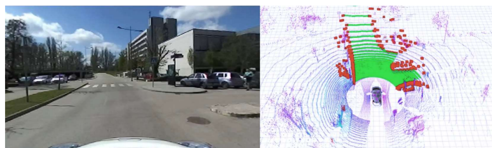
Figure 10. In-vehicle test of the method. On the (left) side, camera information is shown. On the (right) side, LIDAR 3D data are visible where the road (green) and sidewalk (red) are highlighted. The voxel scale is LIDAR intensity-based (location: University Campus, Győr, Hungary).
