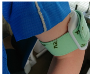
(a) Photograph of wearable device equipped to arm without wearing clothes (the device was covered with clothes in the experiment)
