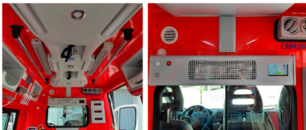
Figure 2. UV-SAN Sanitation Equipment installed in the ambulance patient compartment.
