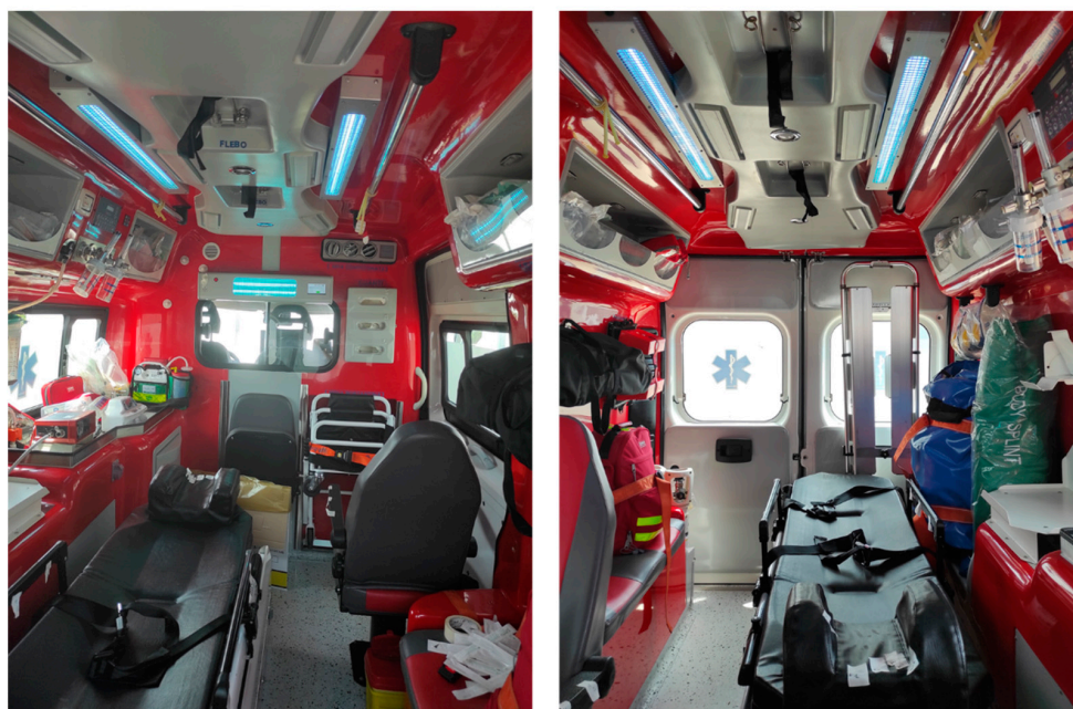
Figure 6. UV-SAN system deployed.
