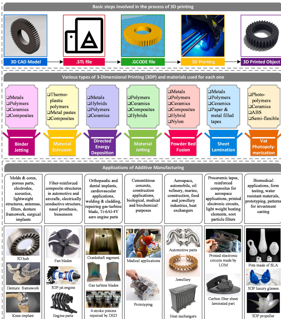
Fig. 3. Schematic, classification, functional materials, and applications of 3D printing.
