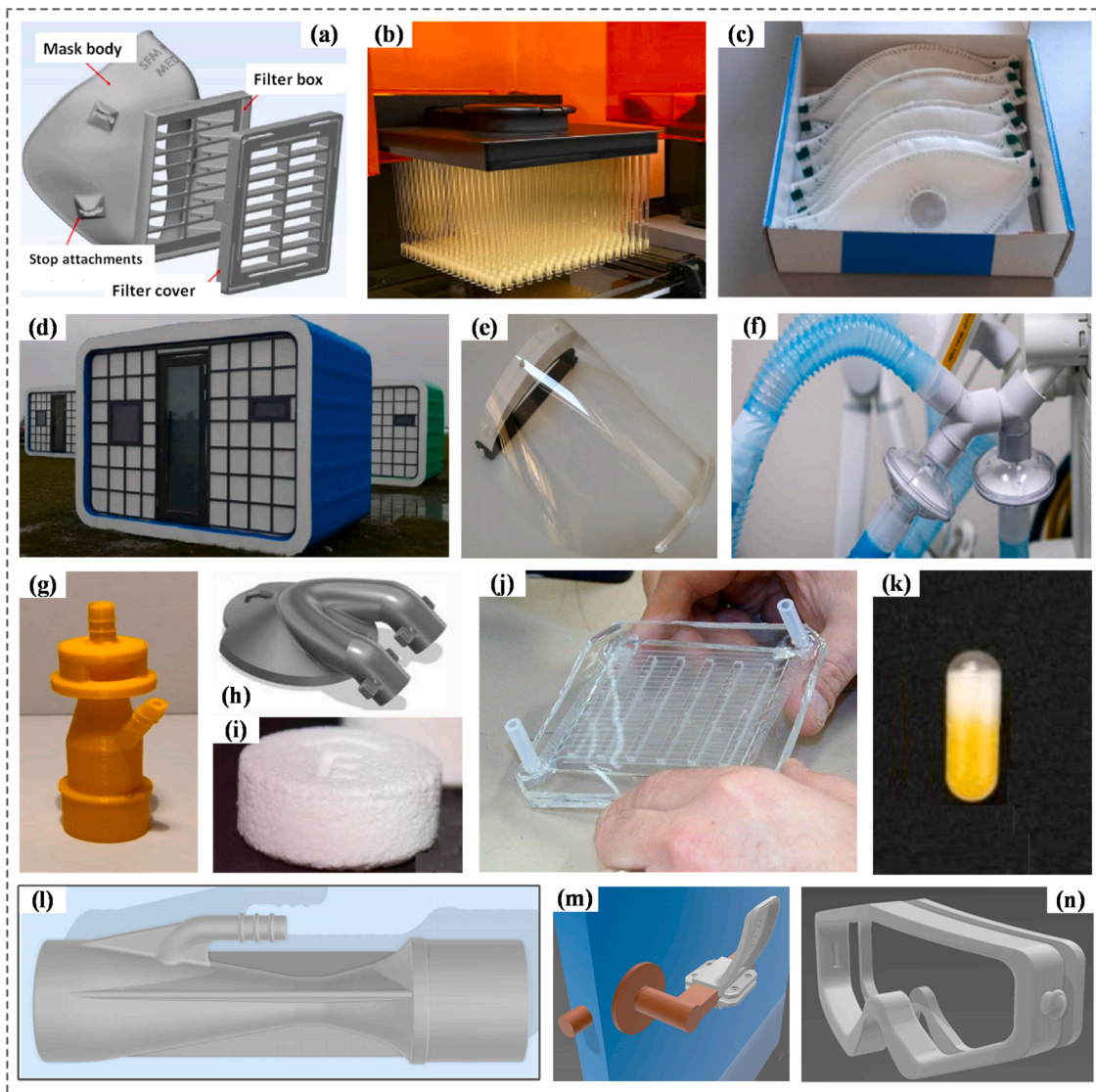
Fig. 13. 3D printed medical devices for applications during pandemic (a) stopgap face mask, (b) swab [16], (c) 3D printed respirator mask [15], (d) quarantine booths [16], (e) face shield, (f) T-connectors, Y-connectors for ventilators, (g) ventilator valve [20], (h) air-purification respiratory hood, (i) 3D printed pills, (j) artificial lung used for lung disease treatment, (k) 3D-printed capsules [14], (l) venturi valve, (m) door handles, (n) Crealitiy goggle design [30].
