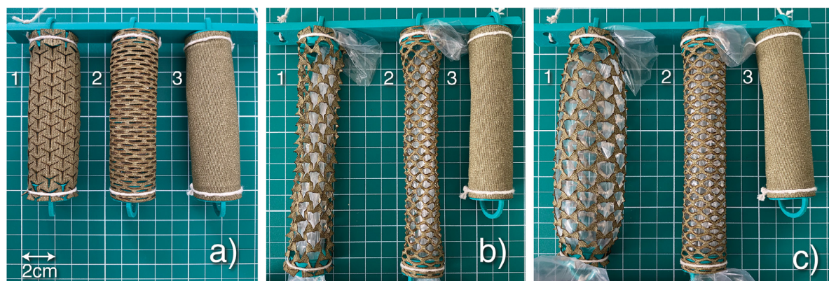
Figure 4. The 3 cylinders used were made of knitted cotton fabric and were each 10-cm long with an 8-cm circumference. Effects of (1) auxetic (star-shaped) and (2) mesh incisions, and (3) no incisions were assessed. (a) Resting state, (b) traction until a length increase of 40% is reached, and (c) an insertion of an inflated balloon inside cylinders with both auxetic and mesh incisions assessed under the same pressure. The control cylinder (3) was not pulled or inflated due to its inelasticity.
