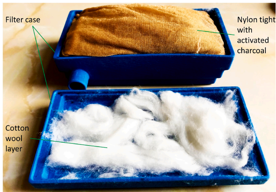
Fig. 7. The 3D printed filter with the filtering material inside.
