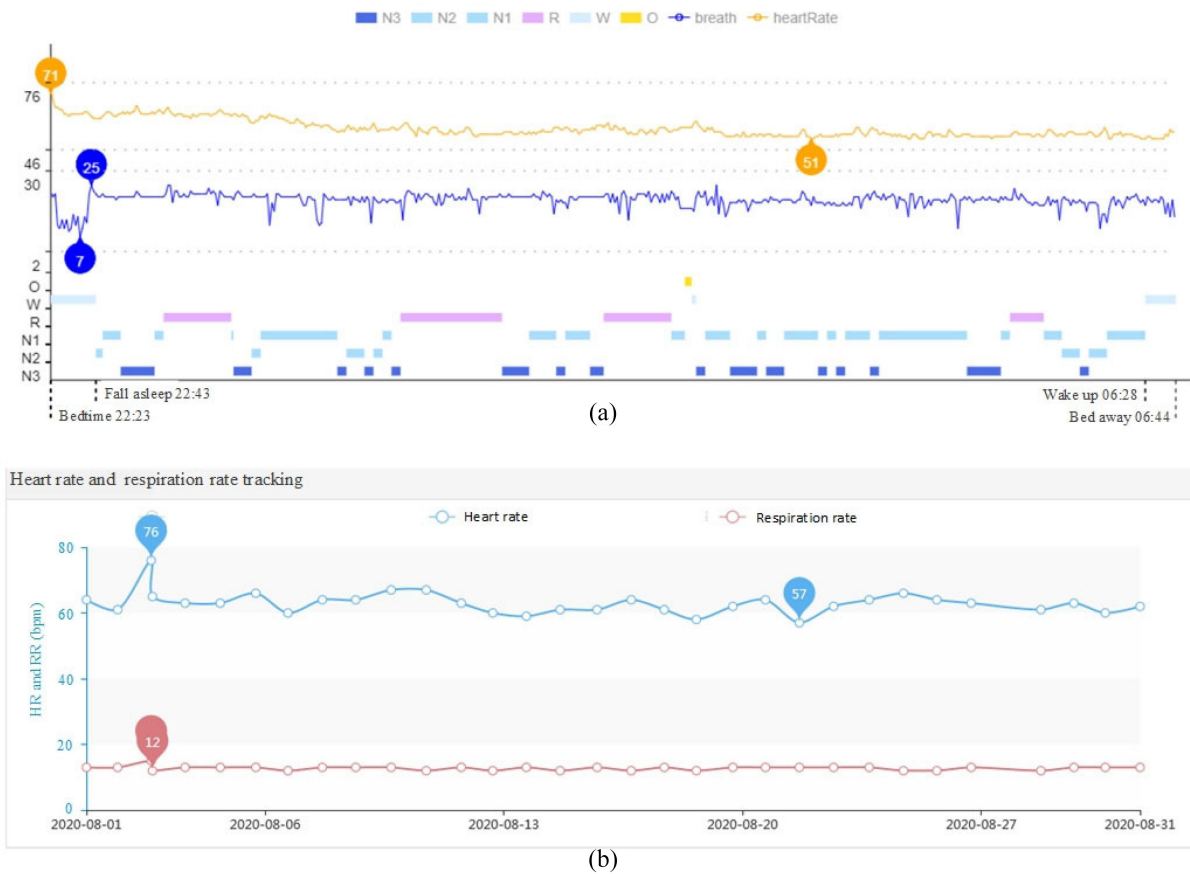
Fig. 10. Example of HR and RR monitoring using the proposed system: (a) continuous monitoring curves of HR and RR at one of the days; (b) benchmark value of HR and RR at each day.
