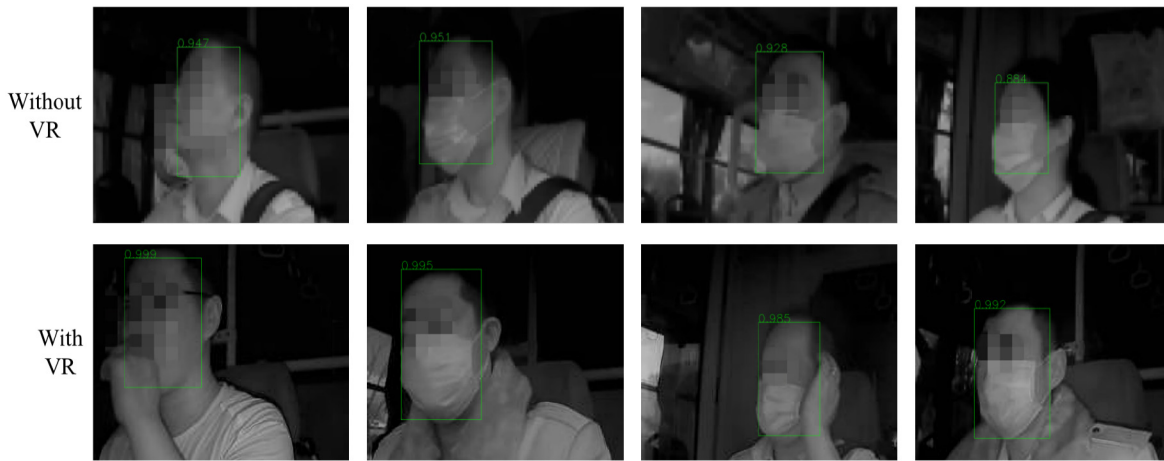
Fig. 5. Visualized results of our face detector with VR and without VR on bus drive monitoring data set, including one Nonmask frame and three masked frames. (Faces portions are pixelated for keep anonymity.)
