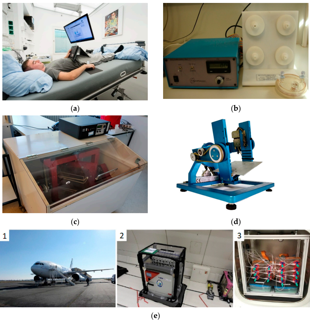
Figure 1. An overview of microgravity analogues. (a) The head-down bed rest experiment configuration (taken from the National Aeronautics and Space Administration (NASA) and Deutsches Zentrum für Luft-und Raumfahrt (DLR), CC BY-NC-ND 3.0 [56]); (b) a commercially available rotating wall vessel; (c) a commercially available three-dimensional clinostat; (d) a commercially available desktop random positioning machine; and (e) experimental setup for a parabolic flight, where image (1) shows the Airbus 310 aircraft used for the parabolic flight, picture (2) shows the incubator used for the experiment, and image (3) gives an impression of the inside of the incubator prior to take off of the flight. The images of (e) were published by Nassef et al. in [57].
