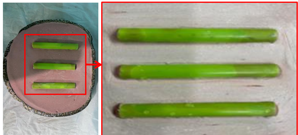
Figure 2. An image for the metal flask with the wax specimens invested and a magnified region of the wax specimen.
