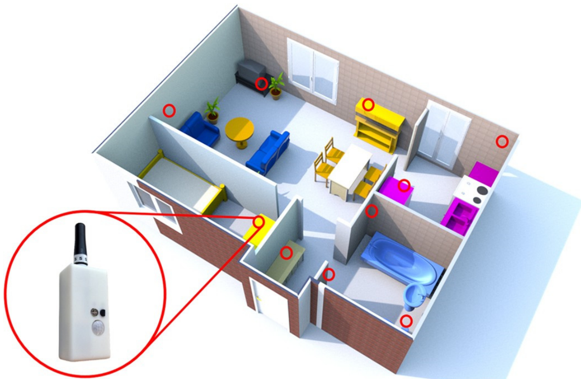
Figure 1. Floor plan of an apartment showing the placement of sensor boxes (red circles). The figure is adapted from Urwyler et al. [30] (CC BY 4.0).
