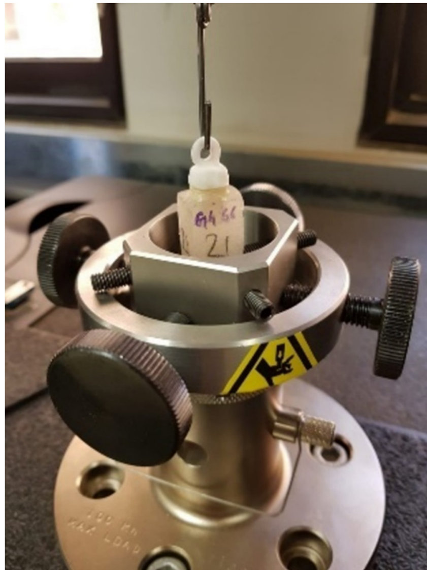
Figure 3. Universal testing machine subjecting copings to dislodgment forces until failure occurred.
