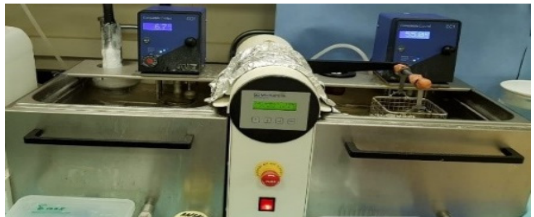
Figure 2. Thermocycling from 5 °C to 55 °C for 3000 cycles using a dwell time of 30 s.
