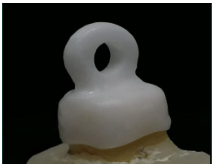
Figure 1. Zirconia coping, designed with a coronal loop (4 mm outer diameter and 2 mm inner diameter) to facilitate tensile loading.
