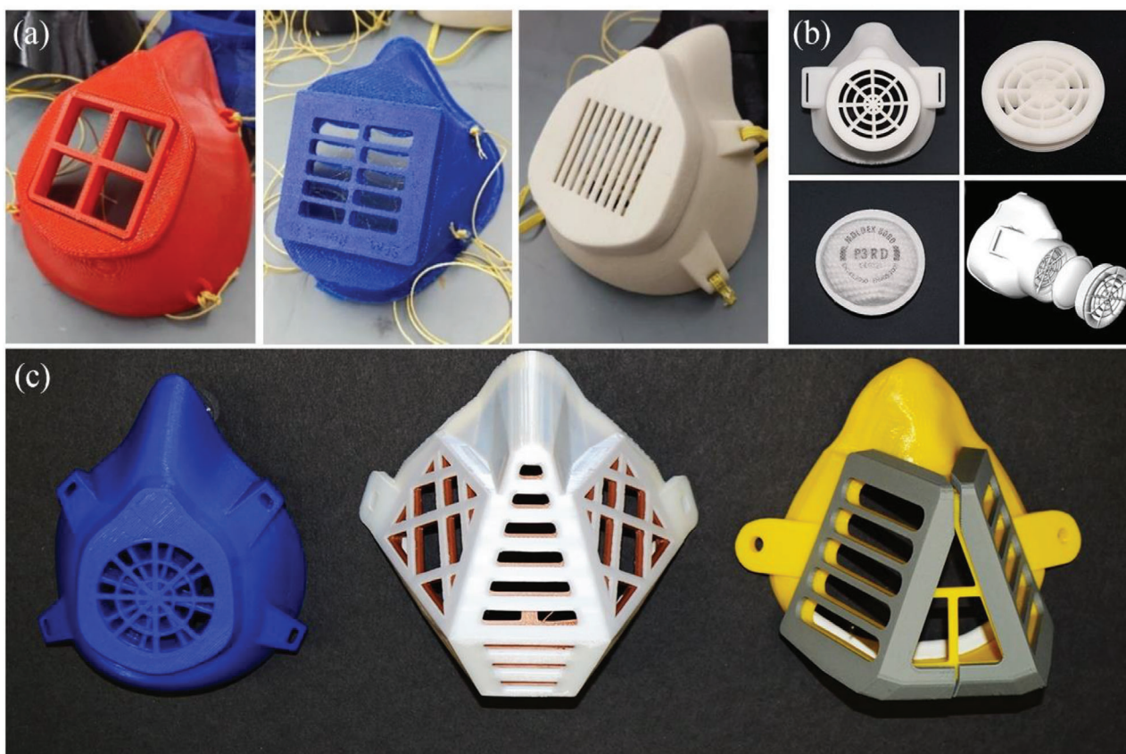
Figure 5. Some examples of 3D-printed masks. a) 3D-printed masks made using open-sourced designs. Reproduced with permission. [132] Copyright 2021, Elsevier. b) A custom-made design for a 3D-printed mask from. Reproduced with permission. [140] Copyright 2020, Elsevier. c) The 3D-printed masks made from PLA using fused deposition modeling (FDM) technology. Reproduced under the terms of the Creative Commons Attribution 4.0 International License. [133] Copyright 2020, Vaňková et al.
