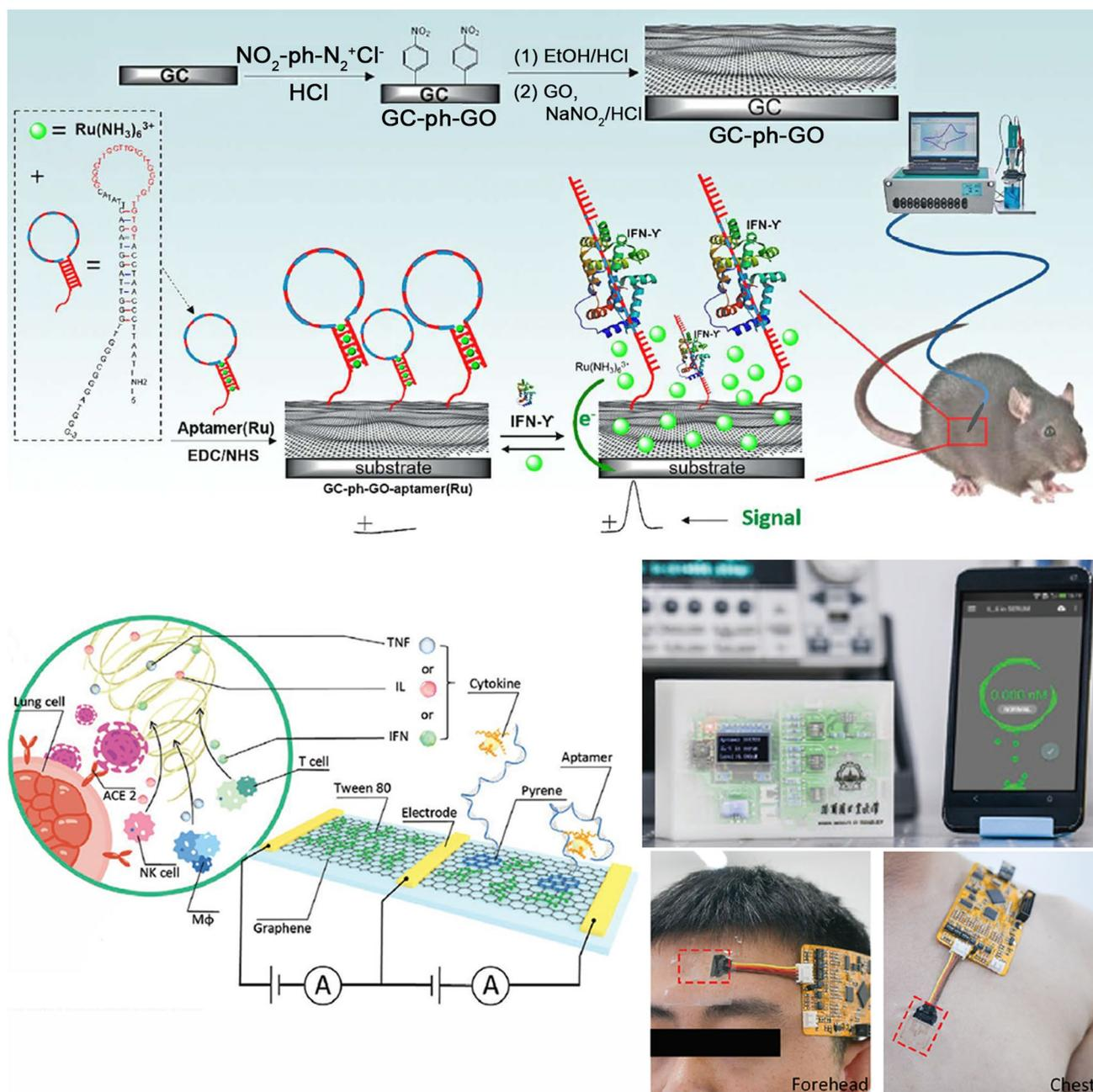
**Fig. 4** Implantable biosensor for the real-time detection of cytokines. When IFN- $\gamma$  binds with the aptamer, it releases ruthenium complexes which generate an electrochemical signal. The device has a low limit of detection and is able to monitor mice in vivo during 48 h. Reproduced with permission from ref. [46] (American Chemical Society
