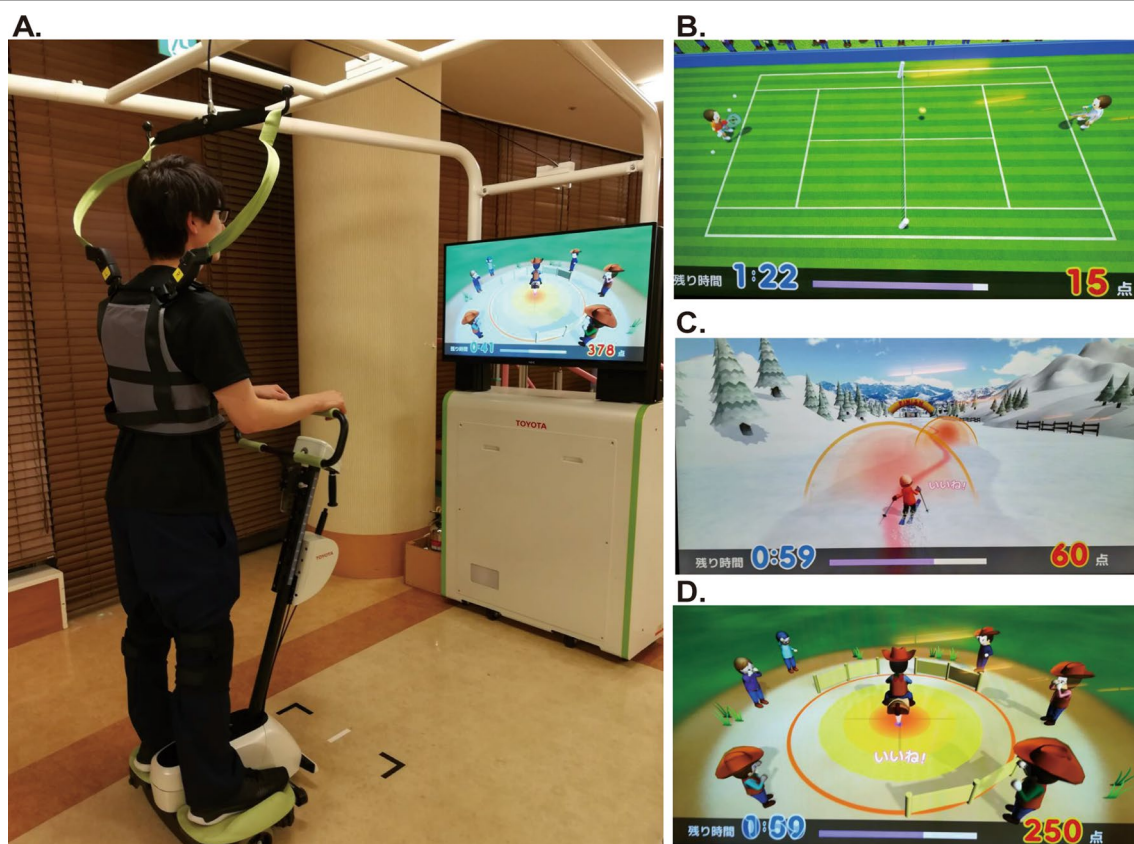
Fig. 1 Balance Exercise Assist Robot (BEAR). A Overview. B Tennis game with active forward and backward center of gravity movement. C Ski game with active left–right weight shift. D Rodeo game in which the patient is required to keep the robot stationary against irregular disturbances
