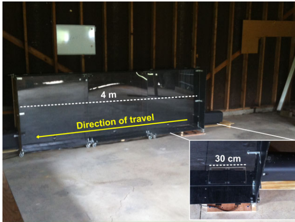
Fig. 4 Custom constructed locomotor runway used for performance testing. Rabbits were coaxed to move across the 4-m-long runway using noxious stimuli (i.e., puffs of compressed air, loud noises, or blunt prods). Inset shows two small animal force plates used to record GRF during trials of burst acceleration. Note that force plates were mounted flush with the runway surface (mechanically isolated from the runway by a gap of 1 cm on all sides) and secured to the floor of the surrounding field station using concrete anchors. Stairway tread tape (3M Corporation, Maplewood, MN) was affixed to the top surface of the force plate to ensure rabbits had sufficient traction for acceleration.
