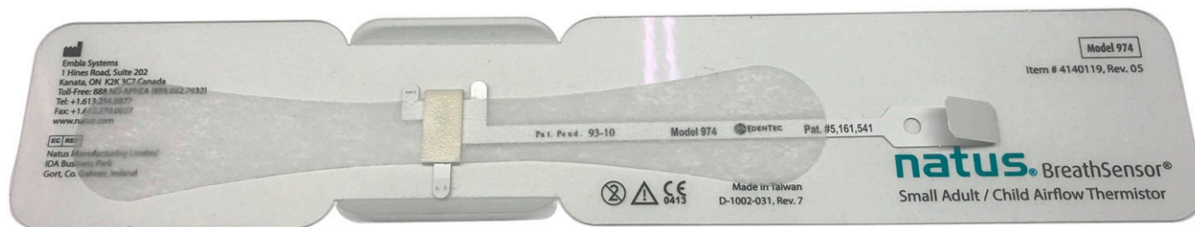
Figure 1 —The Natus Embla BreathSensor airflow thermistor.
