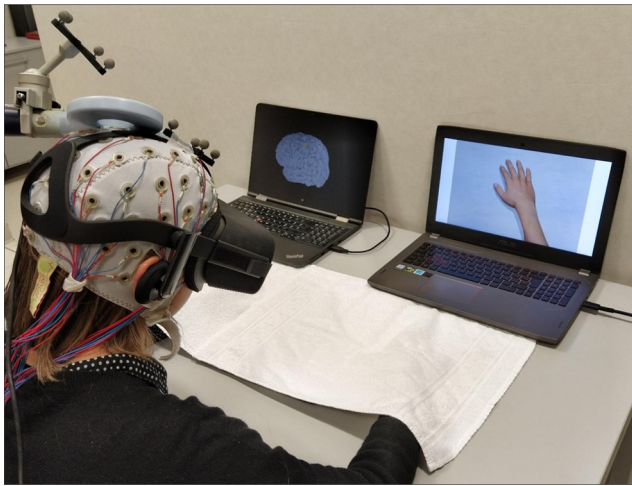
Figure 1. The TMS-EEG-IVR setup. During IVR, each participant was instructed to observe a virtual right hand while TMS was applied over (1) the left ( \text{Wrist}_{l-M1} condition) or (2) the right ( \text{Wrist}_{r-M1} ) hand M1 representation ( M1_{hand} ) or (3) a right disconnected hand while stimulated over the left M1_{hand} ( \text{noWrist}_{l-M1} ). TMS was constantly monitored through stereotaxic neuronavigation, and cortical activation was continuously recorded with EEG. During IVR, participants were asked to refer whether they start to feel the ownership illusion over the virtual right hand, i.e., Sol. TMS, transcranial magnetic stimulation; EEG, electroencephalography; IVR, immersive virtual reality; M1, primary motor cortex; Sol, start of illusion.
