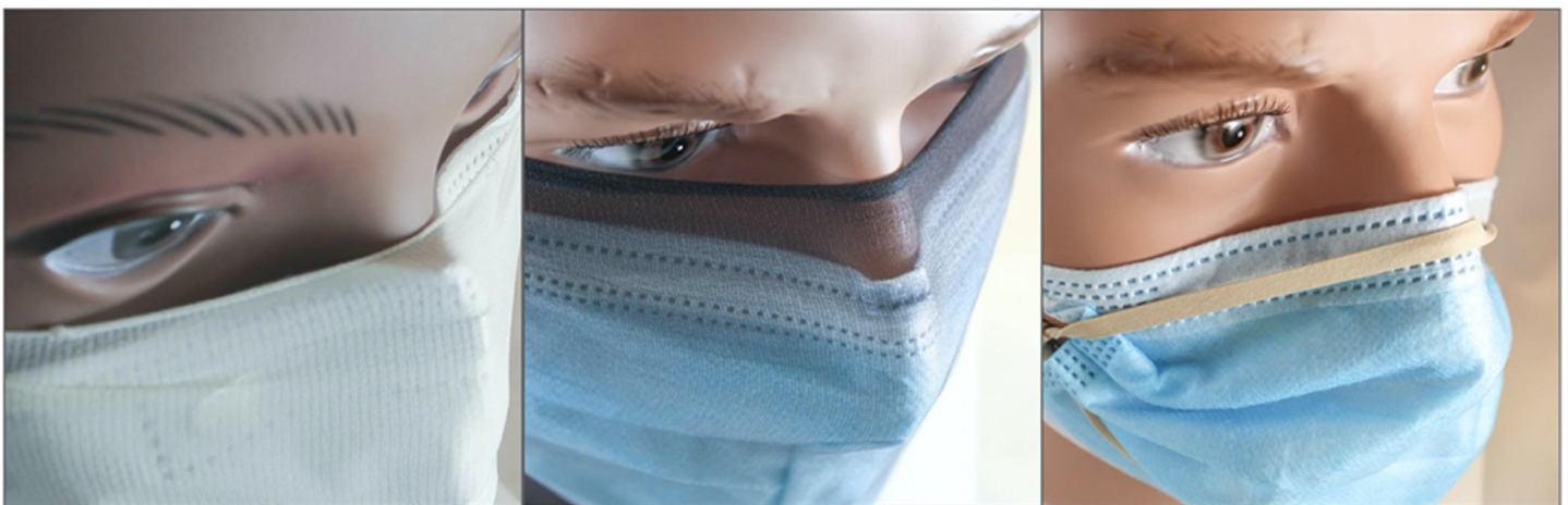
Fig 5. Many fit hacks were unable to fix fit issues around the nose bridge. This impacted wearers with more prominent noses and provided an example of one facial feature critical to the efficacy of fit hacks.
