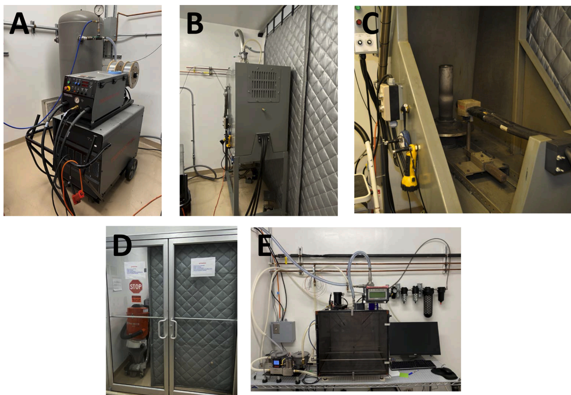
Fig. 2. Images of the completed thermal spray coating generator and exposure system, including the (A) compressed air tank and electric arc wire thermal spray machine with wire feeder; (B) closed spray booth; (C) opened spray booth with spray gun and metal pipe to be coated; (D) glass doors with protective curtains that separates the two rooms of the system; (E) animal exposure chamber with assorted air lines and sampling devices.
