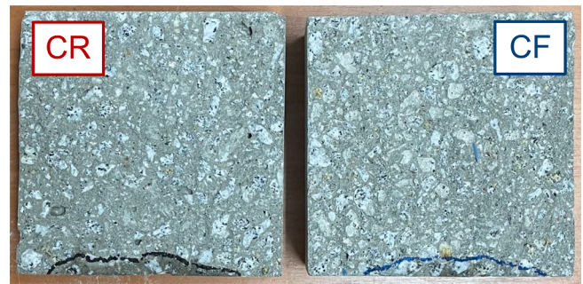
Fig. 7. Exemplary samples after the water permeability test.
