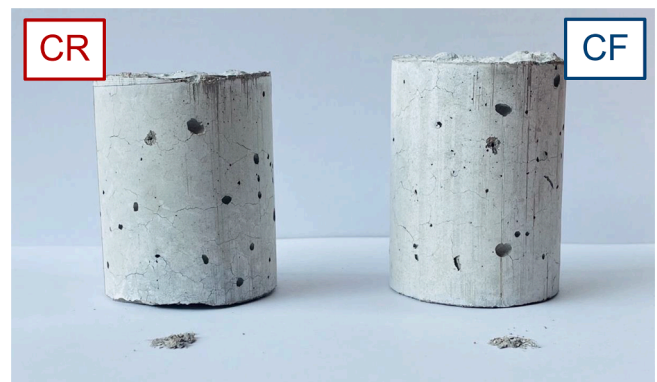
Fig. 8. Exemplary samples after water the spalling test.
