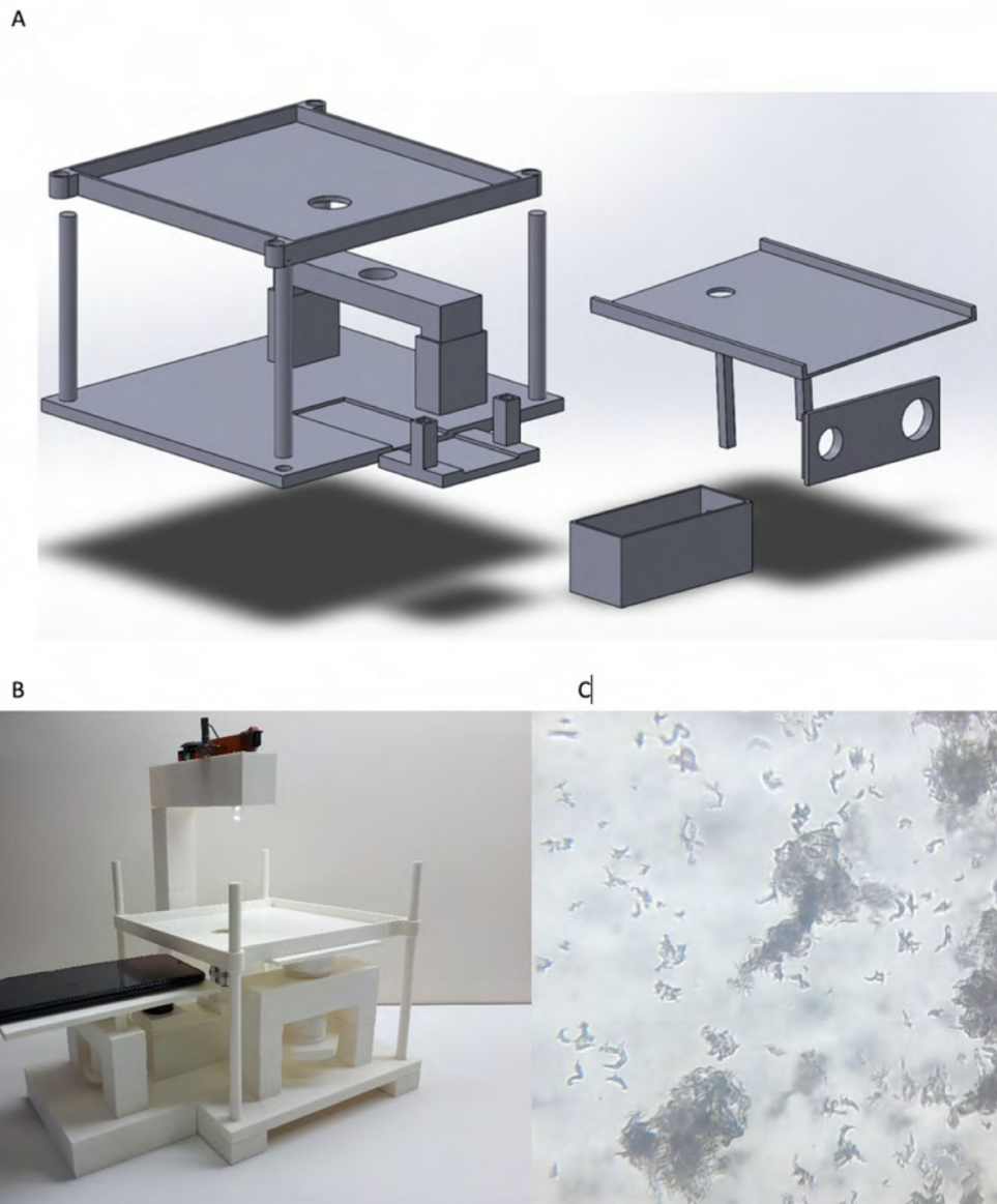
Figure 4: (a) CAD software design of some parts used in the inverted microscope assembly. (b) Inverted printed 3D microscope assembly (c) Image of a 9-day MODS culture taken with the inverted printed 3D microscope.
